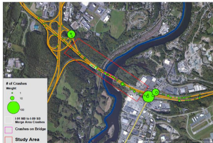
Crashes occur on the I-89 bridges and the adjacent areas.
