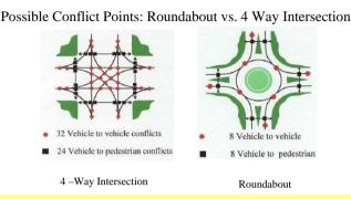
**Safety** – There are fewer conflict points where vehicles can get into an accident in a roundabout as opposed to a 4-way intersection. This combined with the slower speed of vehicles in a roundabout make them very safe.
