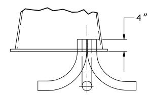
90° ELBOWS - NUMBER, SIZE & TYPE AS REQUIRED IN PLANS OR SPECIAL PROVISIONS. USE STEEL ELBOWS WITH GROUNDING BUSHINGS WHEN CONDUIT RUN EXCEEDS 200'.
