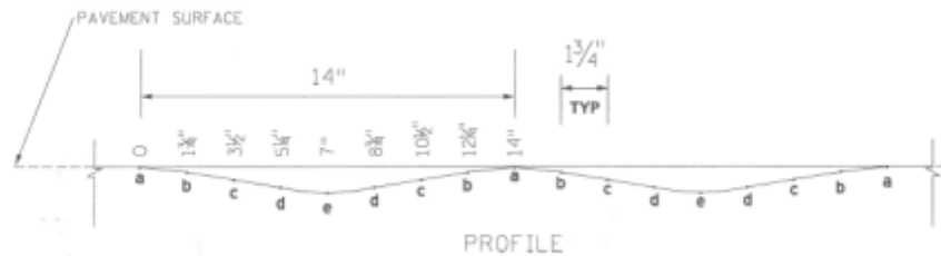
Figure 2. Sinusoidal Rumble Strip - Longitudinal Section
