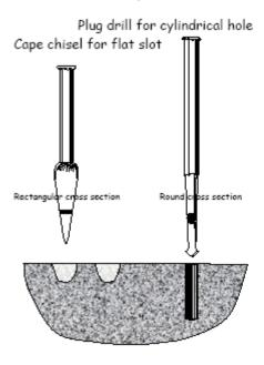
Into this hole were placed a pair of halfround steel shims or "feathers," and between these was driven a wedge or "plug" which exerted outward pressure and split the stone. The advantage of the "plug-and-feathers" method of splitting was the greater depth within the stone at which the wedges exerted their pressure, thus allowing larger pieces to be split more accurately.
