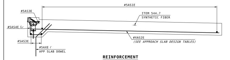
NOTE TO DESIGNER: PROVIDE TOP AND BOTTOM MAT OF REINFORCING STEEL WITH AT GRADE APPROACH SLABS AS USED WITH INTERGRAL ABUTMENTS. OMIT SYNTHETIC FIBER IF BOTH MATS OF REINFORCING STEEL ARE USED.
