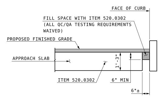
NOTE: DO NOT USE DETAIL WITH APPROACH SLABS FOR INTEGRAL BRIDGES
