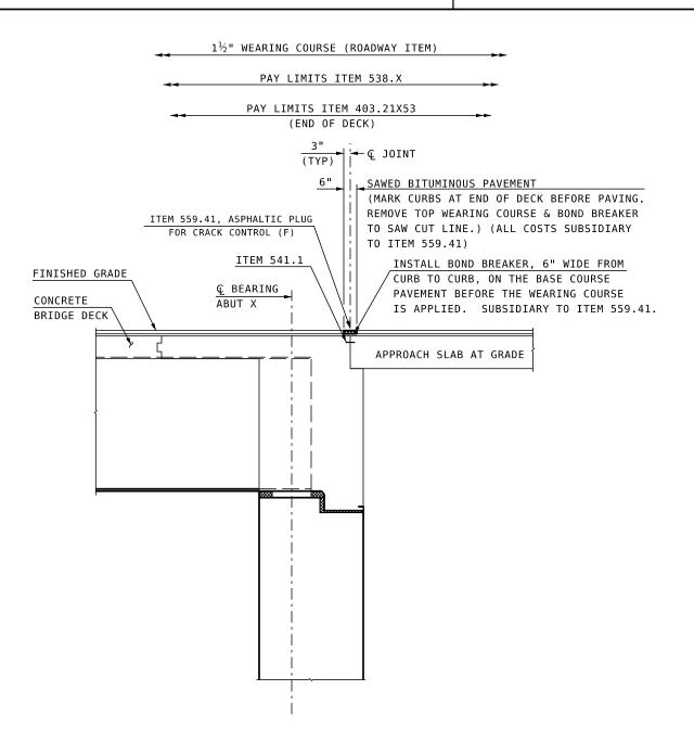
ASPHALTIC PLUG FOR CRACK CONTROL SEMI-INTEGRAL ABUTMENT SECTION
