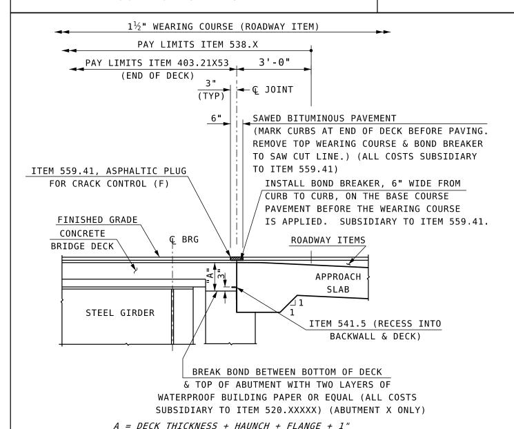
ASPHALTIC PLUG FOR CRACK CONTROL (APPROACH SLAB - FIXED END)
