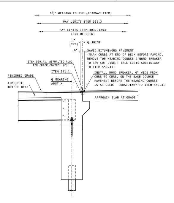
ASPHALTIC PLUG FOR CRACK CONTROL INTEGRAL ABUTMENT SECTION
