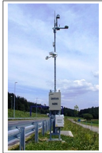
Typical NHDOT Non-Invasive Pavement Sensor System
