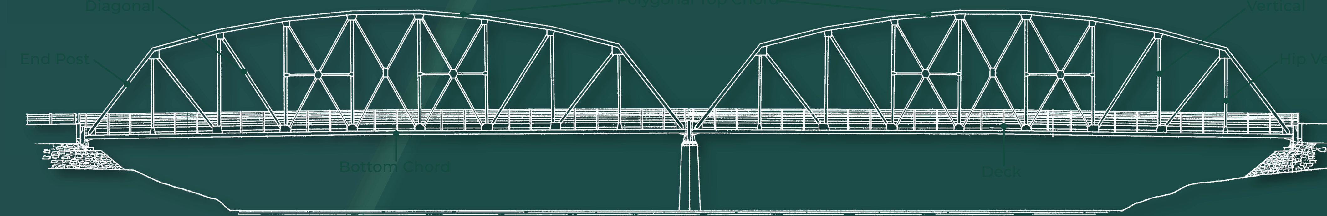
Rogers' Rangers Bridge, General Elevation of the two-span Parker truss bridge of 1950, replaced in 2020. The plans were prepared by the State of New Hampshire, Highway Department Bridge Division, Feb. 1944, revised through Dec. 1949, as it took nearly five years to secure funding.
