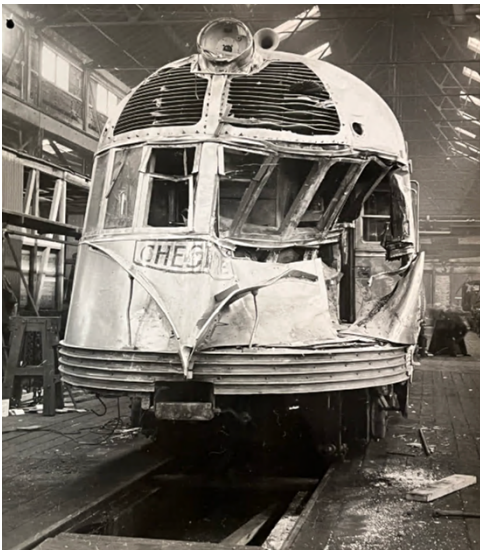
Figure 14. Flying Yankee in the Boston and Maine Railroad repair shops following derailment in January 1945. Source: Boston and Maine Railroad, Maintenance Records.
