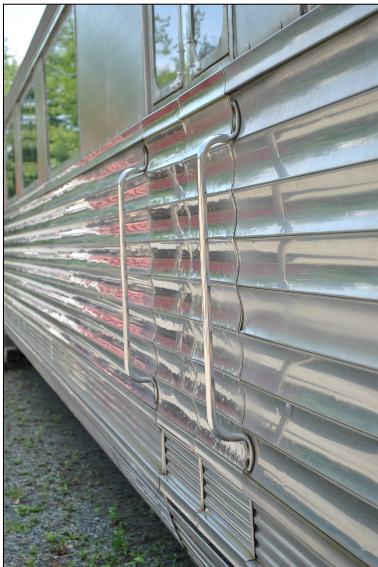
Photo 11. Car B, detail of fluted, stainless-steel, body panels and door handles. View looking south (Patrick Harshbarger, photographer 7/20/23; HRI Neg. #23056 D1:107).
