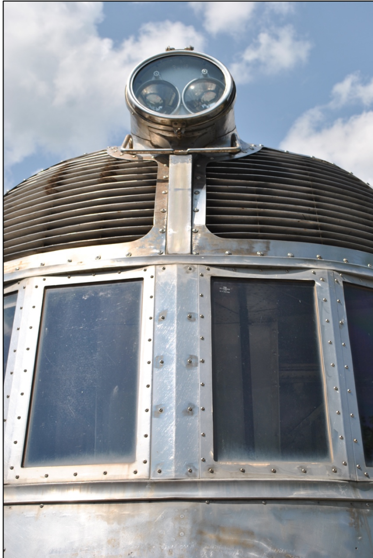
Photo 8. Car A, detail of front headlight, air intake vents and operators compartment front windows. View looking southeast (Patrick Harshbarger, photographer 7/20/23; HRI Neg. #23056 D1:061).
