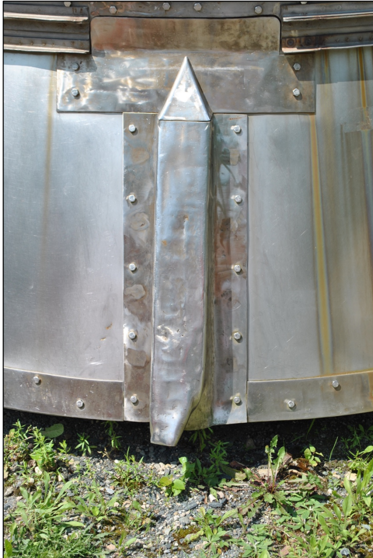
Photo 9. Car A, detail of "cow catcher" and apron at front of train (Patrick Harshbarger, photographer 7/20/23; HRI Neg. #23056 D1:060).
