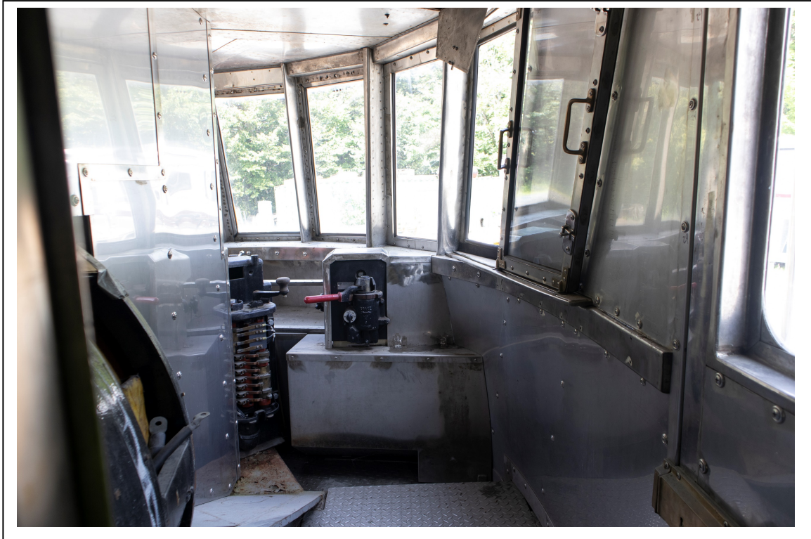
Photo 14 Car A, operator's compartment showing throttle and brake controls, looking northwest toward head of train (Carly Adler, photographer 7/20/23; HRI Neg. #23056 D2:3).
