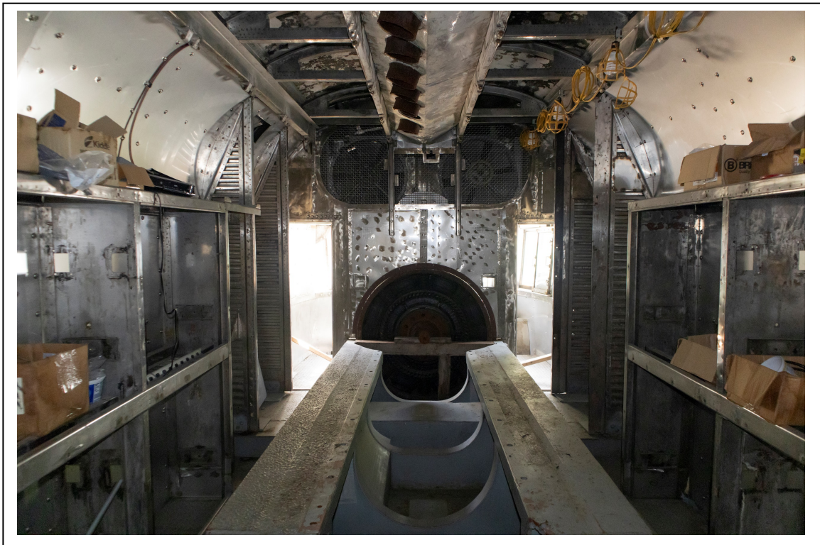
Photo 15. Car A, engine compartment, view looking northwest with cast-steel bed for the diesel engine in foreground (Carly Adler, photographer 7/20/23; HRI Neg. #23056 D2:29).
