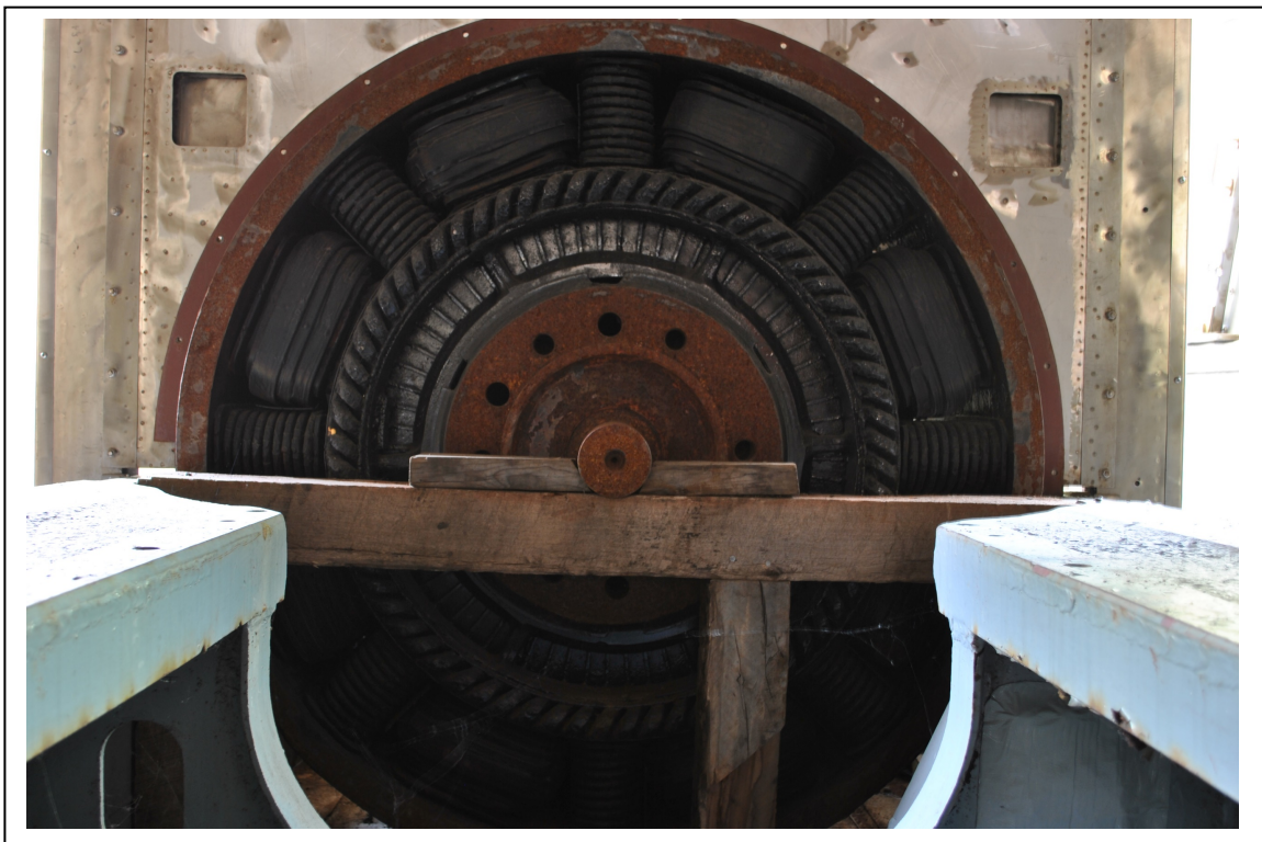
Photo 17. Car A, detail of the main generator at front end of the engine compartment, view looking northwest toward head of train (Patrick Harshbarger, photographer 7/20/23; HRI Neg. #23056 D1:009).
