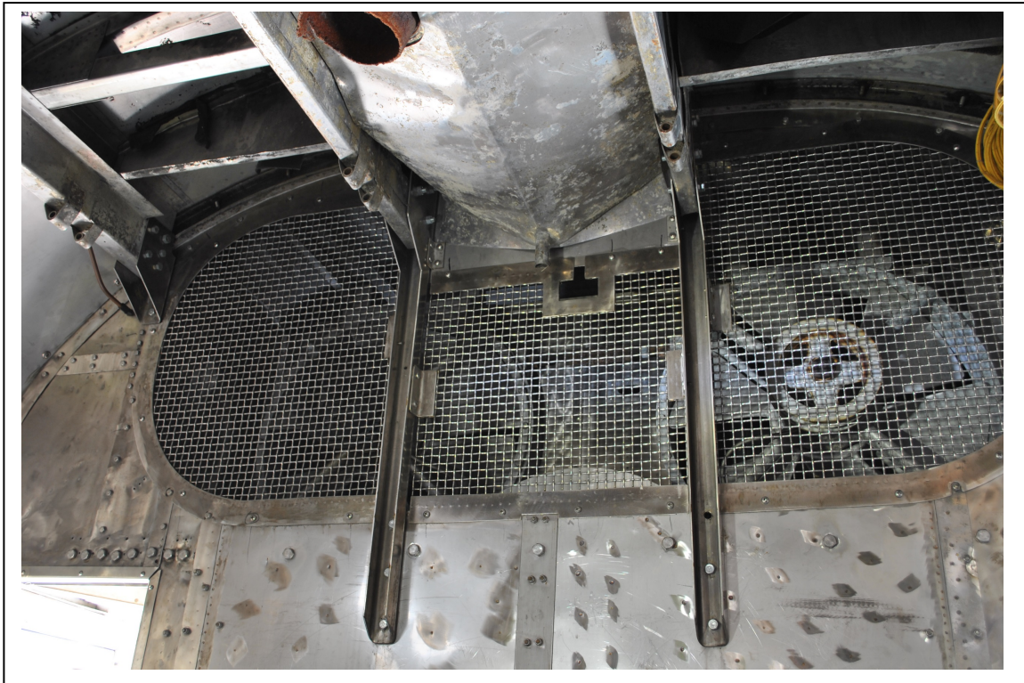
Photo 18 Car A, view of fan housing above the main electric generator at head of train, view looking northwest (Patrick, photographer 7/20/23; HRI Neg. #23056 D1:006).
