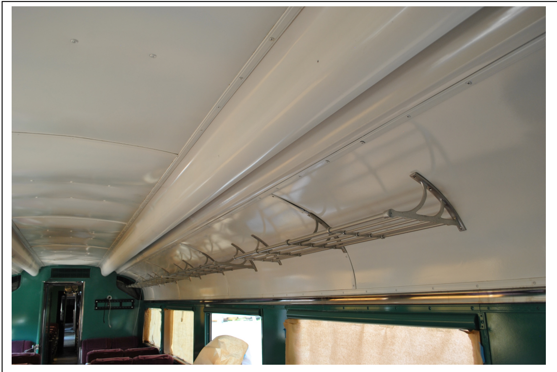
Photo 26. Car B, ceiling detail showing curved lighting shade running length of car and baggage rack. View looking northwest (Patrick Harshbarger, photographer 7/20/23; HRI Neg. #23056 D1:030).
