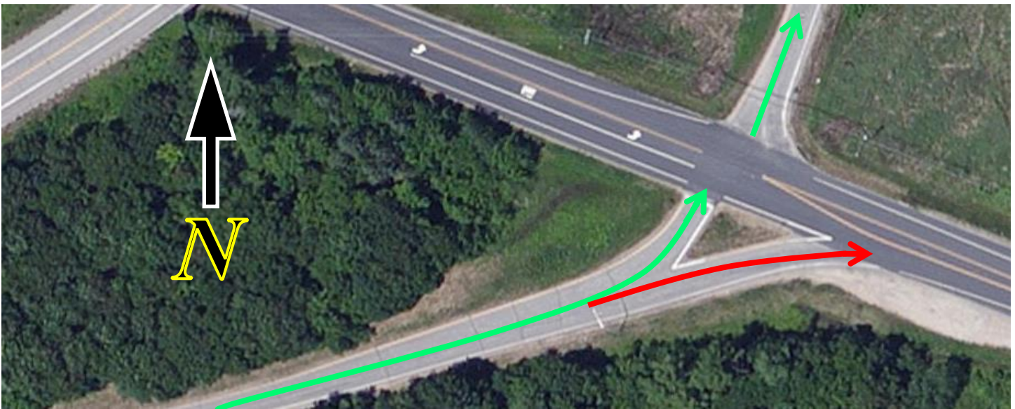
Ramp and slip ramp entering NH 155A from US 4 in Durham, and ramp entering US 4 from NH 155A. The slip ramp (marked in red) diverges from the primary off-ramp, and can only access the eastbound lane of NH 155A. The primary off-ramp (marked in green) can access either direction. Since the on-ramp can be accessed by traffic from either direction on NH 155A, it is classified as a primary ramp, not a slip ramp.
