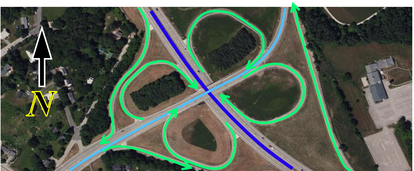
Interchange between NH 16 (shown in dark blue) and NH 9 (shown in light blue) in Dover. Each ramp (shown in green) is not a slip ramp. Despite single directions of access and egress, none of the ramps divide, and are therefore classified as primary ramps rather than as slip ramps, as one might have expected.
